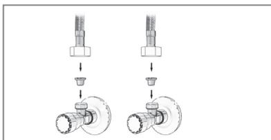
S'ASSURER QUE LES FILTRES SOIENT BIEN PLACÉS ENTRE LES FLEXIBLES ET LES ROBINETS D'ARRÊT (NON FOURNIS)
